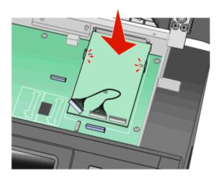
**6** Install the ISP onto the plastic tee. Angle the ISP over the plastic tee, and then approach the plastic tee so that any overhanging connectors will pass through the ISP opening in the system board cage.
