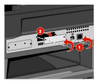
4 Insert the fax card, and then tighten the two screws to secure the fax card mounting bracket.
