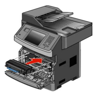
**7** After you replace the photoconductor kit, reset the photoconductor counter. To reset the counter, see the instruction sheet that came with the new photoconductor kit.
