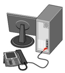
5 Connect an additional telephone cord (not provided) from the computer modem to the printer EXT port m.
