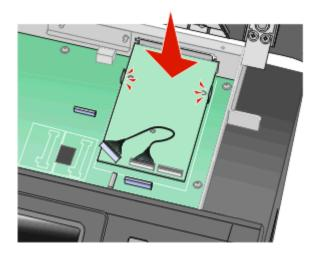
**8** Insert the long thumbscrew, into the hole closest to the white connector, and turn it clockwise enough to hold the ISP in place. Do not tighten the thumbscrew at this time.
