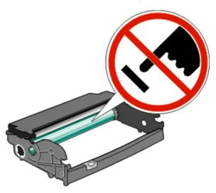
**5** Insert the toner cartridge into the photoconductor kit by aligning the rollers on the toner cartridge with the tracks. Push the toner cartridge until it *clicks* into place.
