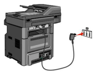
4 If you would like to use the same line for both fax and telephone communication, then connect a second telephone line (not provided) between the telephone and the F slot of an active analog telephone wall jack.
